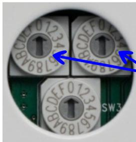
The site code is set in hexadecimal format by the upper two switches located on the rear panel.
